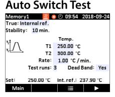
Switch test calibration is a perfect time saver. Start the switch calibration and come back to note the results after the test. You decide if you want the deadband or not - and the test can be repeated automatically in up to three subsequent runs.
