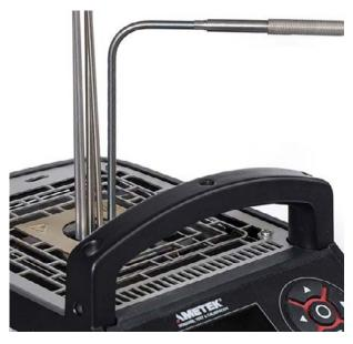
Insert heat loss due to mass loading from multiple or large sensors can be a challenge for most dry-block calibrators.
