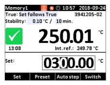
The fastest and simplest way of starting the calibrator. Simply press SET and type in the wanted temperature and off you go.
