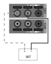
Figure 5 Connection way of Electric Current(mA) Measurement
