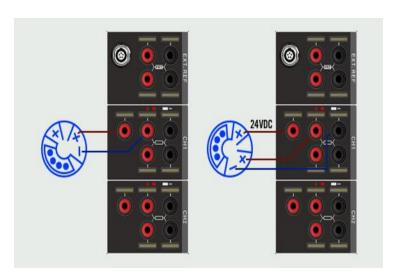
Figure 8 HART Transmitter Connection Diagram
