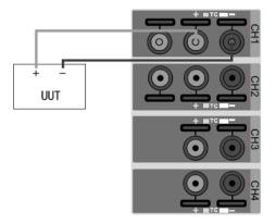
Figure 6 Connection Diagram for Voltage Measurement
