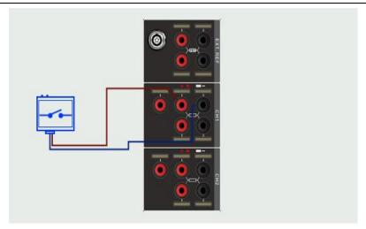
Figure 7 Connection Diagram for Switch Testing
