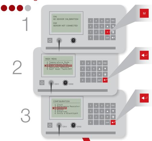
SENSORS 1 New/Edit Calibr. 2 Delete Calibr. • 3 Select Sensor #1 4 Select Sensor #2 CH1 SN SELECT SENSOR No: 014V Ç CH1 CH2 SAVE CHANGES +1 YES 2 NO Ç СН1 СН2
