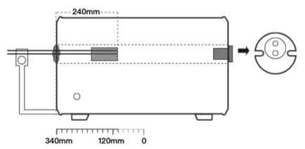
Figure 2-12 Base metal + short furnace + cup design insert
