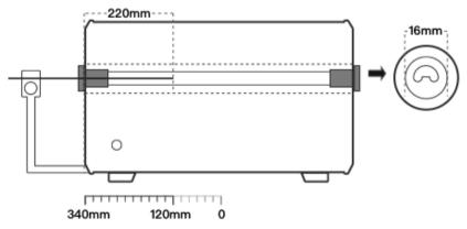
Figure 2-14 Noble metal + φ16mm alumina tube
