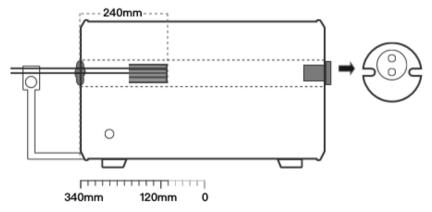
Figure 2-13 Base metal + short furnace + multi-hole design insert
