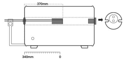
Figure 2-9 Base metal + long furnace + multi-hole insert
