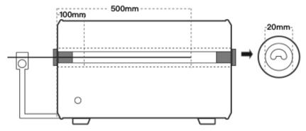
Figure 2-10 Noble metal + long furnace + φ20mm alumina tube
