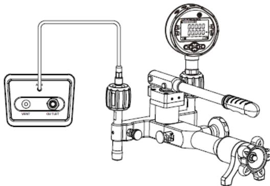
Figure 4- 1 Calibrate an barometric pressure module
