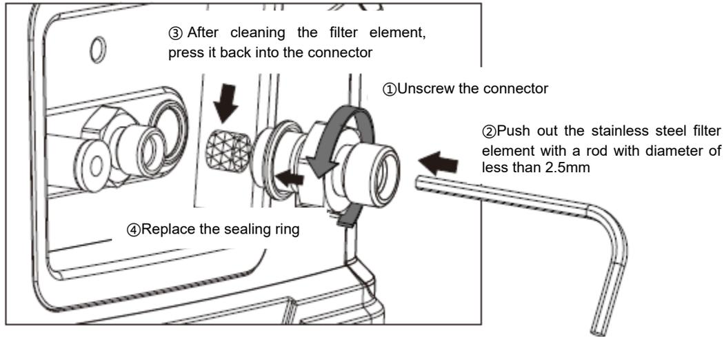
Figure 8- 3 Disassembly of differential pressure connector
