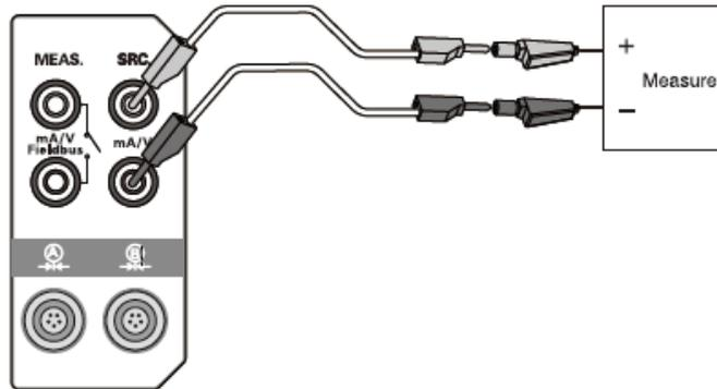
Figure 3- 10 Current output of internal power supply
