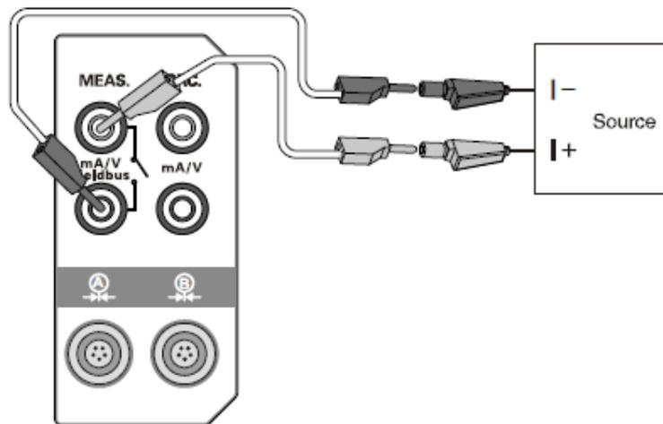
Figure 3- 5 Current measurement
