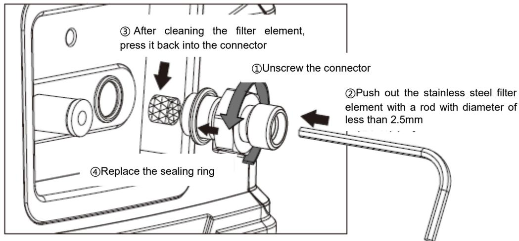
Figure 8- 2 Disassembly of high-precision/barometric (BP) version pressure connector
